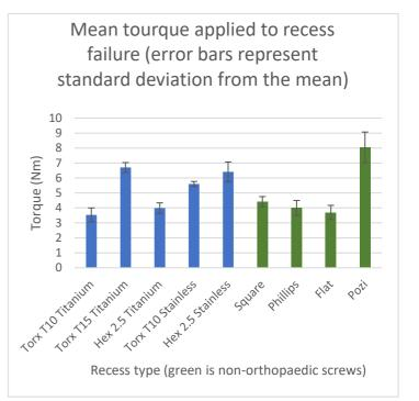
**Discussion:** There are multiple factors that contribute to recess failure. including the type of metal used, characteristics of the screw head, in our study the highest torque was observed in the stainless steel pozidriv screw heads. Although, the best orthopaedic screw tested was the titanium T15 torx, it is likely that a stainless-steel version would perform the best, thus decreasing risk of metalware removal.
